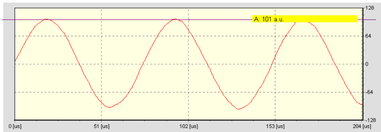
Figure 63. Measurement of the detected signal produced from phase detector. To increase the measurement dynamic (and accuracy) measure peak-to-peak value rather than peak.
