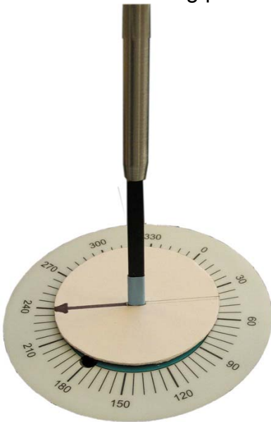
Figure 76. Tesla meter probe and the hand made disc assembly on the magnet's dial.
