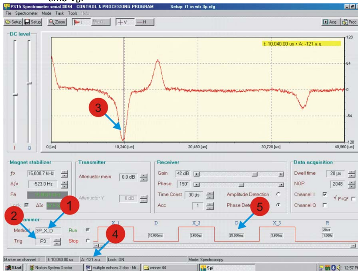
Figure 108. For T_1 measurements select and use the 3P_X_D method (1), set triggering after P3 pulse (2), place measuring cursor on the center of stimulated echo (3). Due to short relaxation the third secondary echo is not visible.
